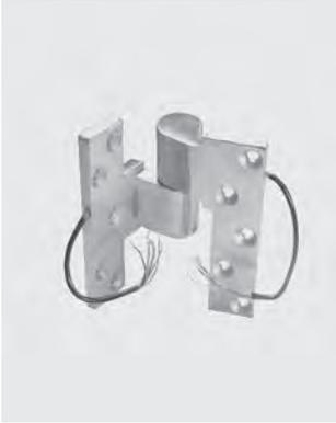
**75200**—Electrified intermediate pivot for power transfer. This eight-wire design uses #28 AWG, rated for 24 V maximum. Pairs of wires connected together provide 2 amps maximum. Multiple pairs provide greater amperage ratings, i.e. two pairs in a circuit provide 4 A maximum, and four pairs provide 8 A maximum. Pivot is non-load bearing and has non-separable pivot leaves. Specify Hand.
