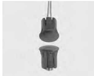
**MC-4**—Self-locking recessed mount. 3/4" dia. magnetic contact. Accommodates up to a 1/2" gap between the door and frame.
