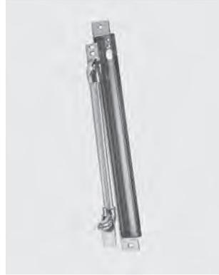
**ES105**—Power transfer with steel housing and flexible tube. Secure and inconspicuous channel to bring power from frame to door. Narrow, shallow channel easily mortises into door edge. Accepts up to 5/16" dia. wire bundle. Accommodates doors that swing open 120°. Concealed when door is closed. Suitable for wood, aluminum, or steel applications.
